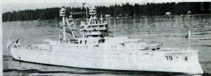
Builder: Cecil/Pat Gates, Lake Almanor, CA. Hull: Fiberglass, Power: 2 OMC Saildrives. Laid Down: August, 1982. Launched: July 3, 1984. Scale: 20:1. Pilot: Driven from conning tower — 345° view. Length: 34 ft. Beam: 6 ft. Draft: 2 ft. USS Arizona (BB-39) "Flagship," Battleship Division, 1941. Builder: N.Y. Navy Yard. Launched: 19 June 1915. Laid Down: 16 March 1914. Cost: $12,993,579.23. Length: 608 ft. Beam: 97 ft.
